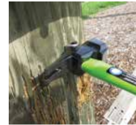
Integrated removable staple puller
